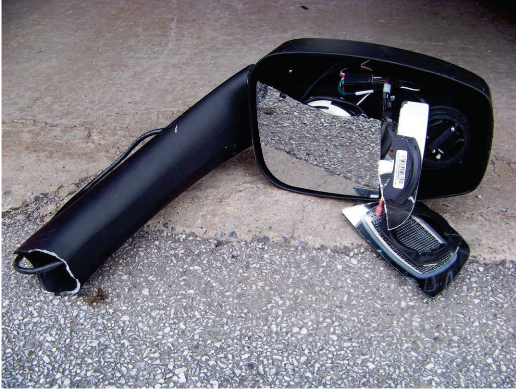
CURBSIDE MIRROR ARM SNAPPED (681 TEST MILES)
