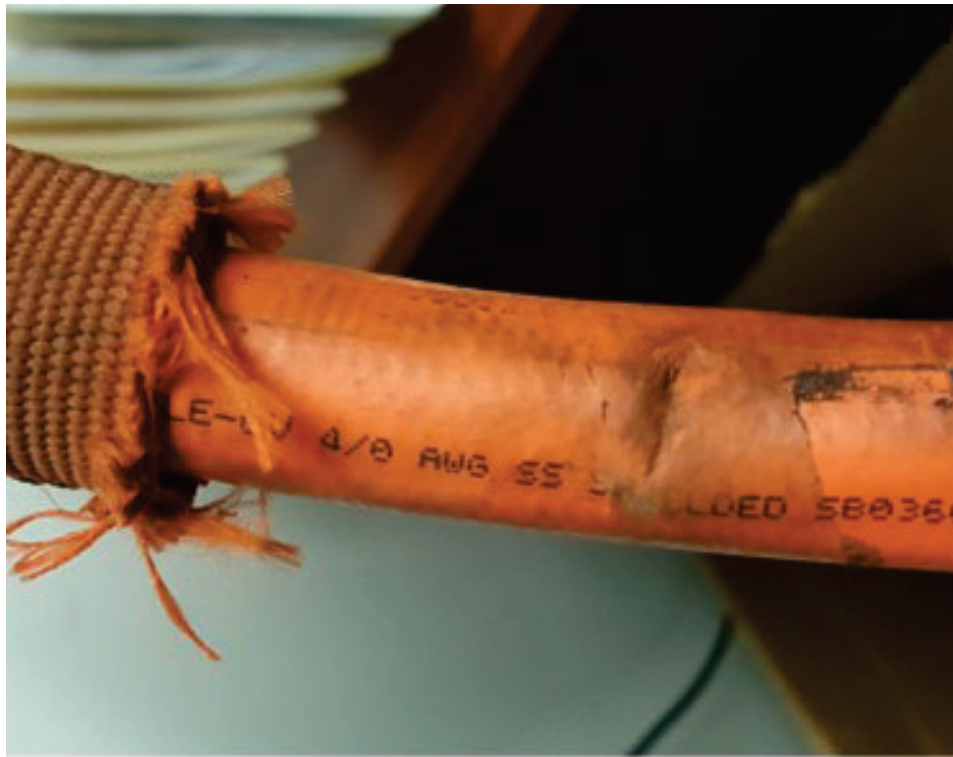
DAMAGED DC CABLE GOING TO DUOPOWER AXLE (2,669 TEST MILES)
