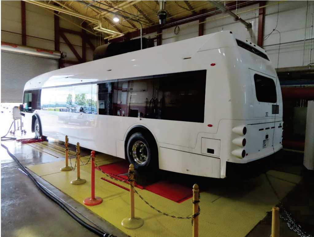
BUS TESTED ON CHASSIS DYNAMOMETER FOR PERFORMANCE AND ENERGY ECONOMY
