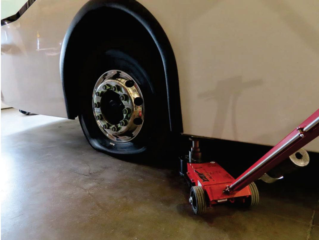
JACK IN PLACE – FRONT
