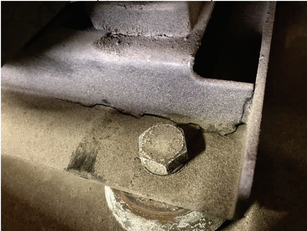
AIR COMPRESSOR BRACKET IS CRACKED (12,598 TEST MILES)
