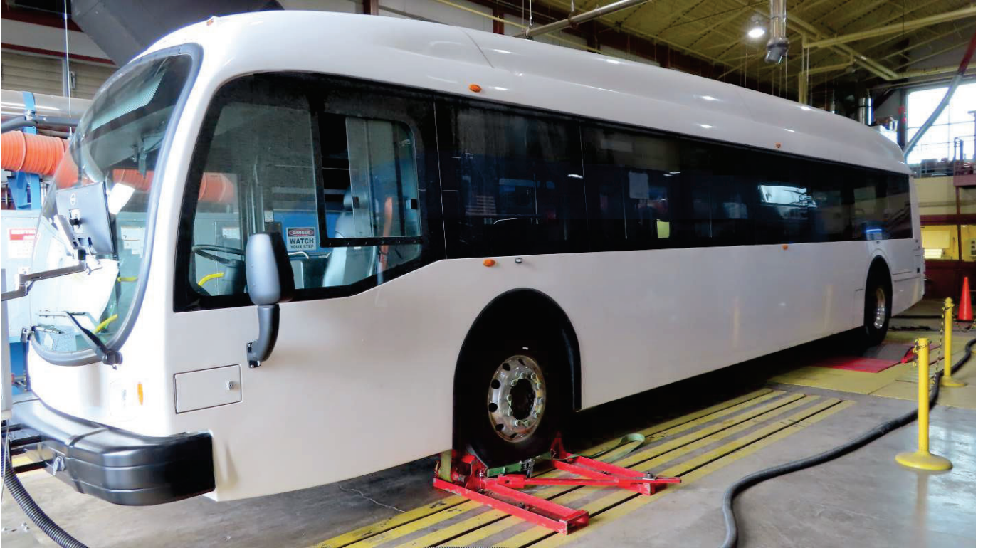
BUS TESTED ON CHASSIS DYNAMOMETER FOR PERFORMANCE AND ENERGY ECONOMY
