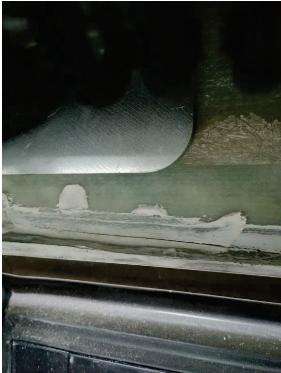
CRACKS AROUND REAR DOOR (12,999 TEST MILES)
