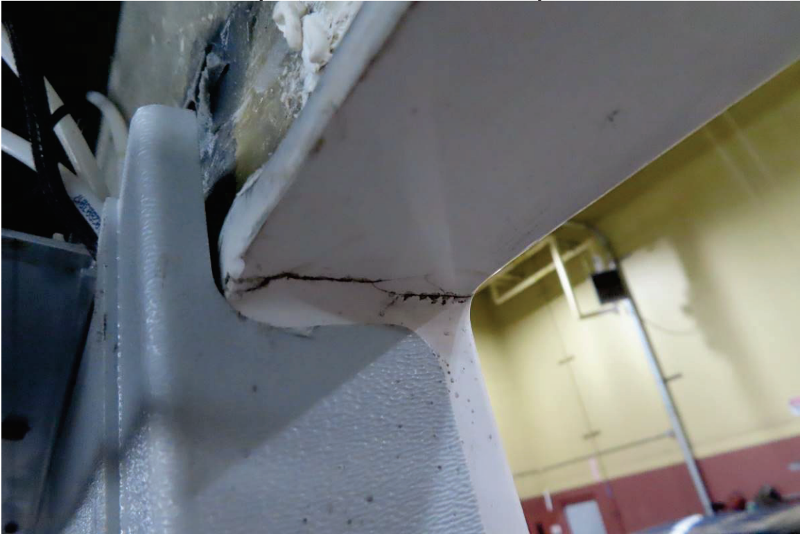
CRACKS AROUND REAR DOOR (12,999 TEST MILES)
