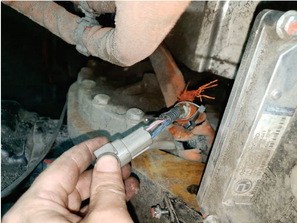
SHIFT POSITION SENSOR WIRE IS BROKEN (1,648 TEST MILES)
