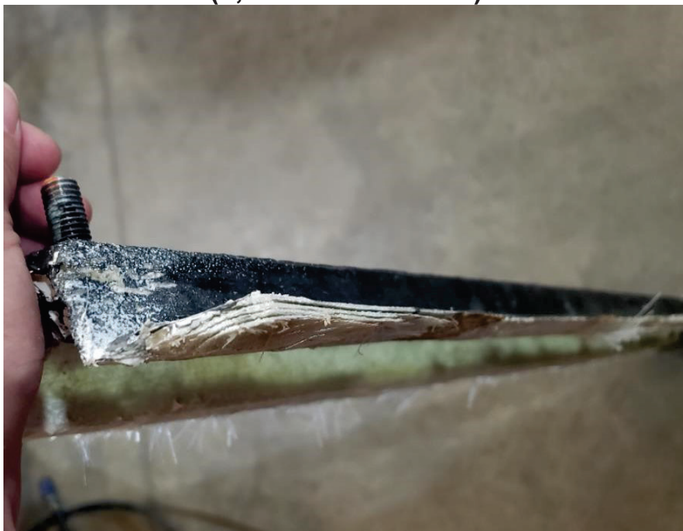
DAMAGED FRONT DOOR HAT BRACKET (6,494 TEST MILES)
