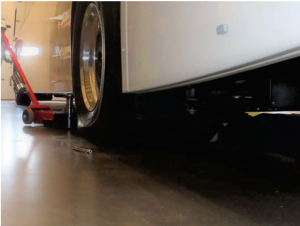
JACK IN PLACE – REAR
