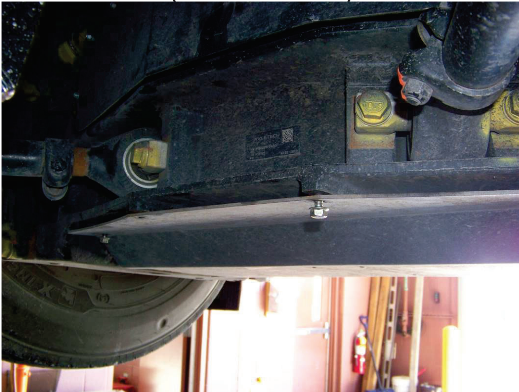
BOLTS LOOSE ON REAR AXLE COVER (755 TEST MILES)
