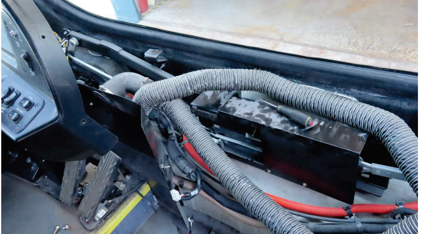
DASH PIECES REMOVED TO ACCESS WIPER MOTOR
