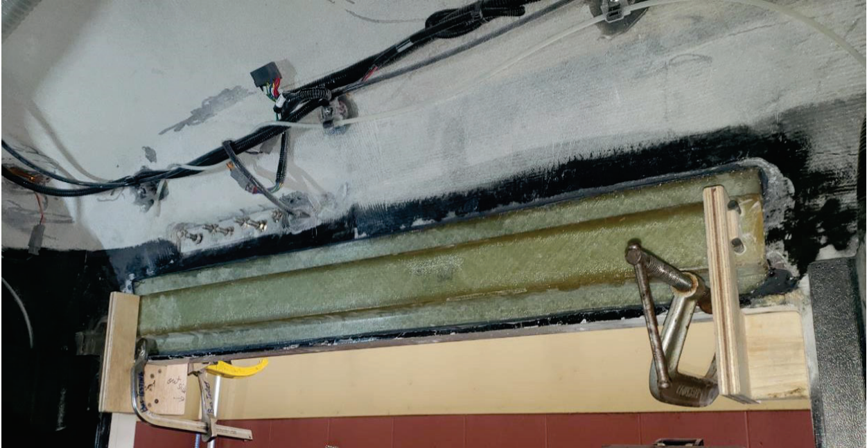
FRONT DOOR HAT BRACKET REPAIR (6,494 TEST MILES)
