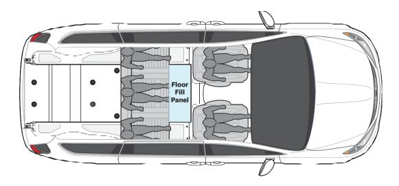
\*\*\* These floor plans to include a three-passenger bench seat in second row \*\*\*
