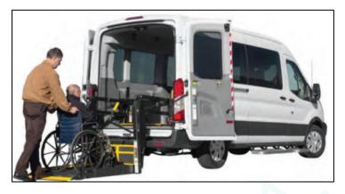
Body on Chassis Vehicle with Lift (14-, 15-, and 19-passenger; can be customized to include more wheelchair tie downs and reduce overall passenger count)
